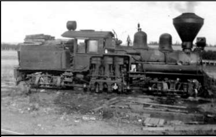
Figure 5: One of the two Class B Shays owned by the Deer Lumber Company. The Deer Park Lumber engine roster lists two such locomotives with the Lima engine #2219 having built on October 12, 1909. This picture was taken in September 1920. (Photograph from the Lawrence Zimmer Collection)
