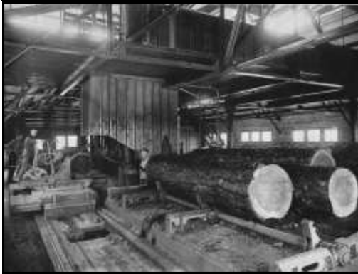
Figure 7: The Clark Brothers' band saw mill in action with the sawyer in the light colored shirt and the setters riding the carriage. (Photograph courtesy of the Deer Park Open Door Congregational Church)
