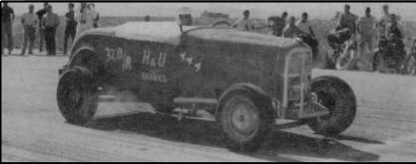
Figure 3: Bud Prufer and Charles Geisler's 275 cubic inch Mercury powered 1932 Ford Roadster. It won the B roadster trophy in the "Safari" race with ease with a top speed of 94.43 miles per hour. (Photograph taken from page 25 of the September 1955 Hot Rod Magazine)
